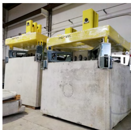
40Tn Handling equipment for Ondraf/Niras IPM (Installation for the production of monoliths) in Belgium
